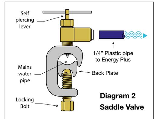
**WATER SUPPLY PRESSURE MUST NOT EXCEED 100 PSI.** This is not a problem if using mains water. Failure to set correct pressure could result in leakage/bursting of unit.
